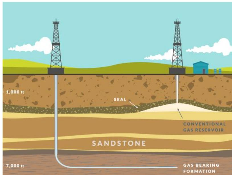
**Figure 6.1:** A horizontal well drilled through a tight shale (Left) and a conventional, vertical well drilled into a porous sandstone reservoir (Right) (Crone, 2015).
